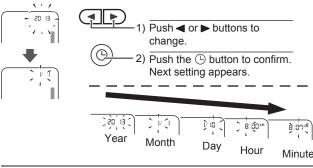
3. Press the START/STOP button to store the setting. • If the batteries have been replaced, the date and time setting will need to be reset. • If the date and time are not set, "-:--" appears during or after
