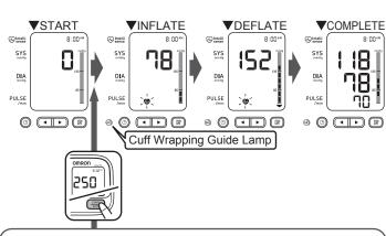
If your systolic pressure is more than 210 mmHg After the arm cuff starts to inflate, press and hold the START/STOP button until the monitor inflates 30 to 40 mmHg higher than your expected systolic pressure.
