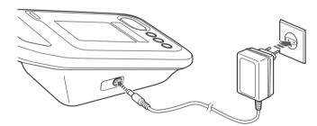
Connect the AC adapter to the DC jack on the unit and the power outlet.
