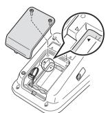
4. Replace the battery cover and secure with screws.
