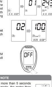
If the meter is left idle for more than 5 seconds after entering the memory mode, the meter then will display the following message on the LCD and the strip indication light will flash.
